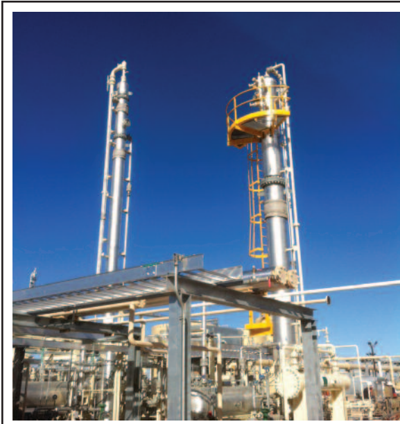
A patented refrigerated fractionation system was developed to recover natural gas liquids from the carbon dioxide-reinjection streams in tertiary oil recovery operations. The process plants for the new NGL recovery method typically cost between $500 and $700 an Mcf, depending on location and gas composition.
